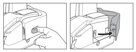
**2** Dampen a cloth with water, wring the cloth out thoroughly, and then wipe off the dirt around the ink absorber.
